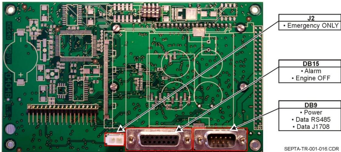
**Figure 37 — KC640 CPU Board (Part Number 0404B, Rear View)**
