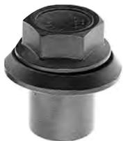
2-piece, 78.5 mm height, 33mm hex head flange nut. Mounts dual wheels with 32mm bolt holes to wheel centering hubs. Right hand threads used on both sides of vehicle. P/N 430732; M22x1.5 RH threads.
