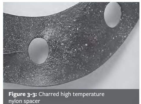
Figure 3-3: Charred high temperature nylon spacer
