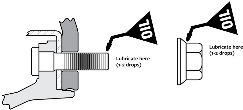
Prior to mounting hub piloted wheels, coat the wheel hub bore. Then push wheels onto the hub so that excess lube will scrape off and not be pushed between the mounting surfaces with a non-water-based lubricant to minimize corrosion and build-up between the wheel and hub pilot. Excessive corrosion build-up between the wheel and hub pilots can make wheel removal difficult. Do not lubricate the face of the wheel, hub or brake drum.
