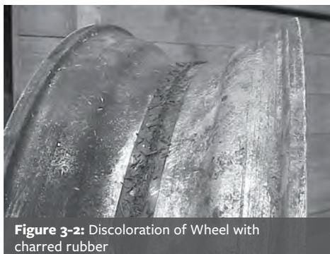
Figure 3-2: Discoloration of Wheel with charred rubber
