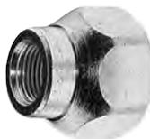
3/4"x16 cap nut. Mounts standard single wheels and wide base wheels to 3/4" studs. Do not use on steel wheels. P/N 5995R, 5995L (replaces P/N 5554R, 5554L).
