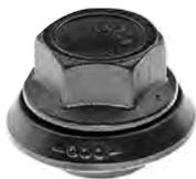
2-piece, 50mm height 33mm hex head flange nut. Mounts single wheels to wheel centering hubs with 32mm bolt holes. Right hand threads used on both sides of vehicle. P/N 430632; M22x1.5 RH threads.
