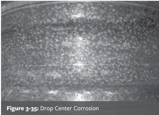
Figure 3-35: Drop Center Corrosion
