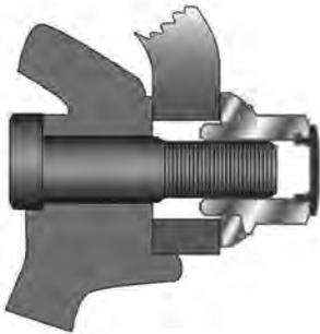
Single mounted wheels require sleeved flange nuts with a short sleeve.
