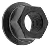
2-piece, 26.25 mm height, 33mm hex head flange nut. Mounts single and dual wheels to wheel centering hubs. Right hand threads used on both sides of vehicle. P/N 39874 (supersedes P/Ns 39701 and 39691); M22-1.5 RH threads.
