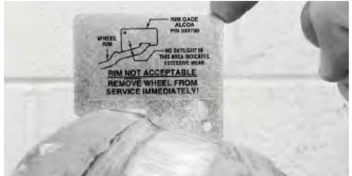
Figure 3-27: Not serviceable (scrap wheel)
