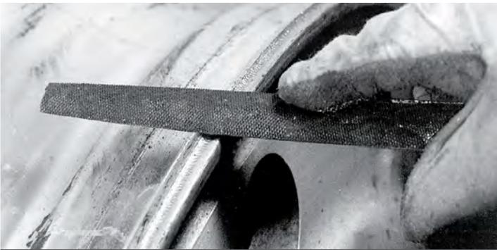
Figure 3-30: Removing sharp edge by hand with a metal file.
