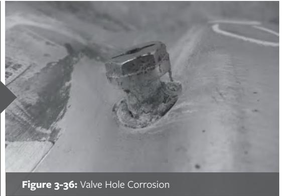
Figure 3-36: Valve Hole Corrosion
