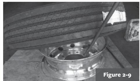
For aluminum wheels, a mat should be placed on the floor to prevent damage to the mounting surface of the wheel.
