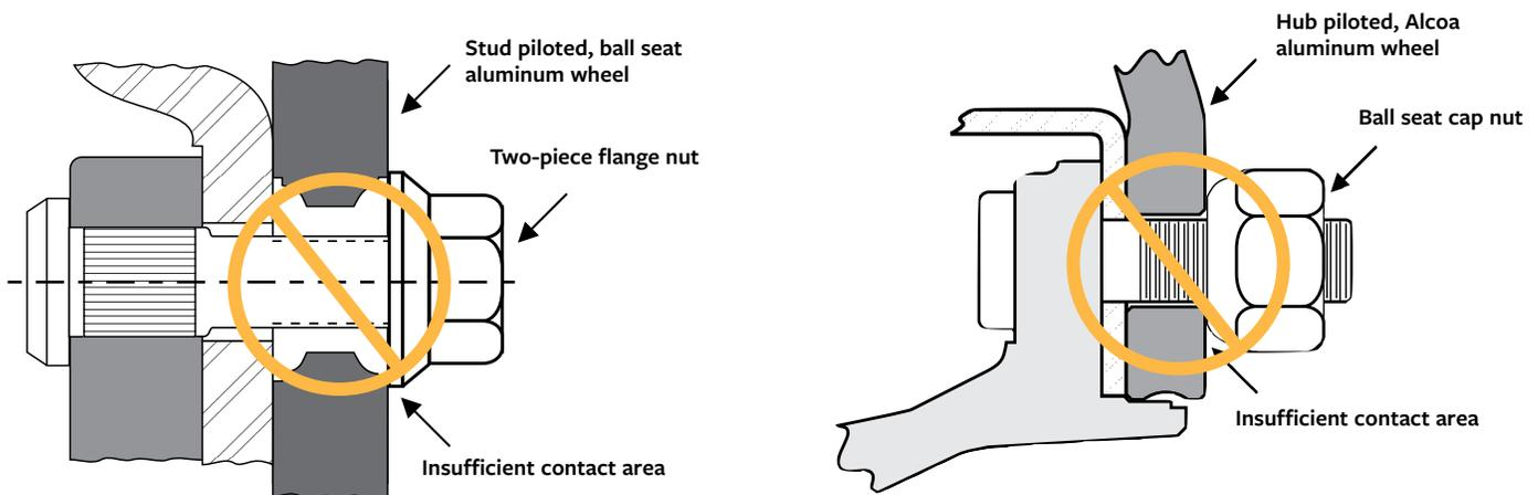
Incorrect use of a ball seat cap nut on a hub piloted system. Do not use ball seat cap nuts with hub piloted wheels.
