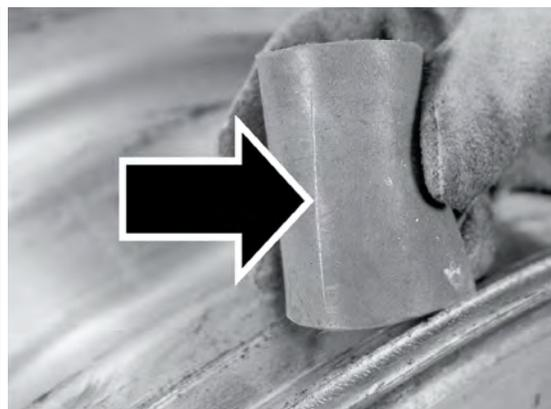
Figure 3-29: Run the sharpness indicator gauge along the wheel in the area of the wear to determine if the wear is sharp enough to cut or damage the rubber on the sharpness indicator.
