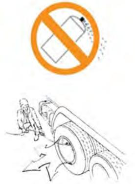
If ANY of these conditions are present — STOP! DO NOT approach tire. Before removing from OSHA compliant restraining device, completely deflate tire remotely. Remove clip-on air chuck. Mark tire as damaged for a potential “zipper rupture” (render tire immediately unservicable, non-repairable and scrap).
