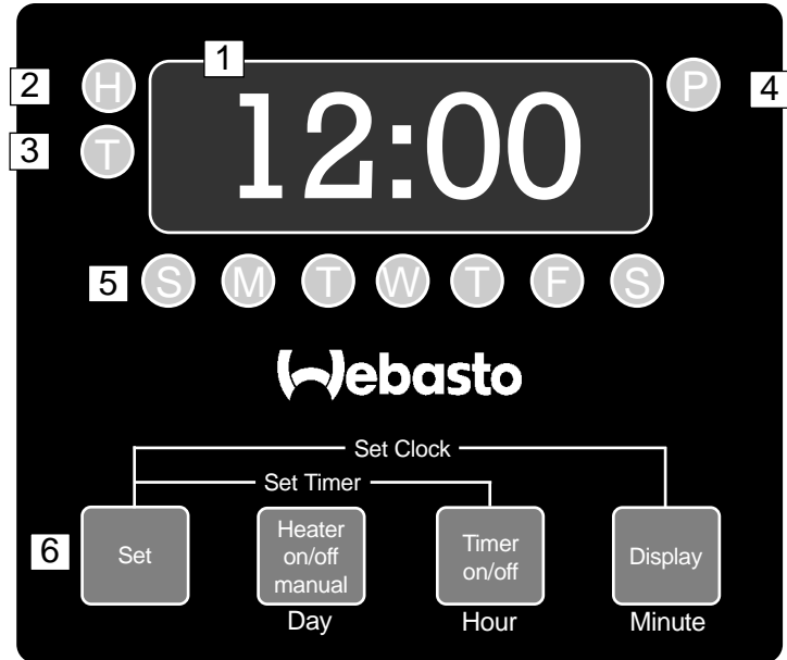
Fig. 5: 7-Day Electronic Timer Model CDN-1224
