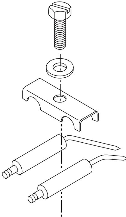
Figure 43: Ignition Electrode Replacement
