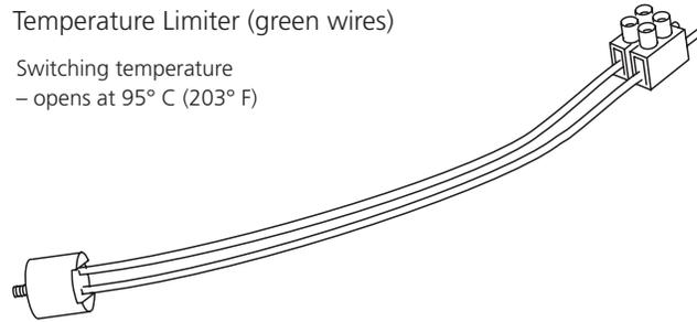
Temperature Limiter (green wires)
