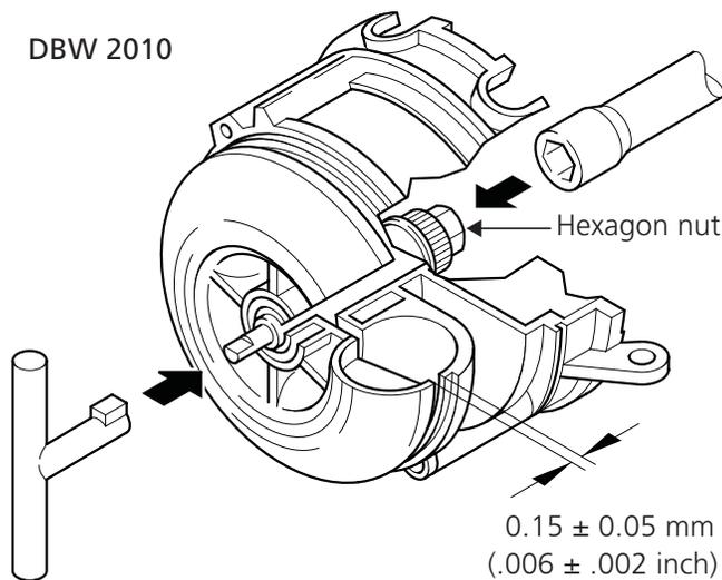
Figure 35: Clearance Adjustment - DBW 2010 Fan
