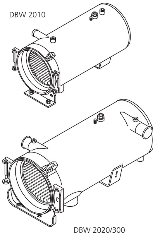
Figure 17: Heat Exchangers
