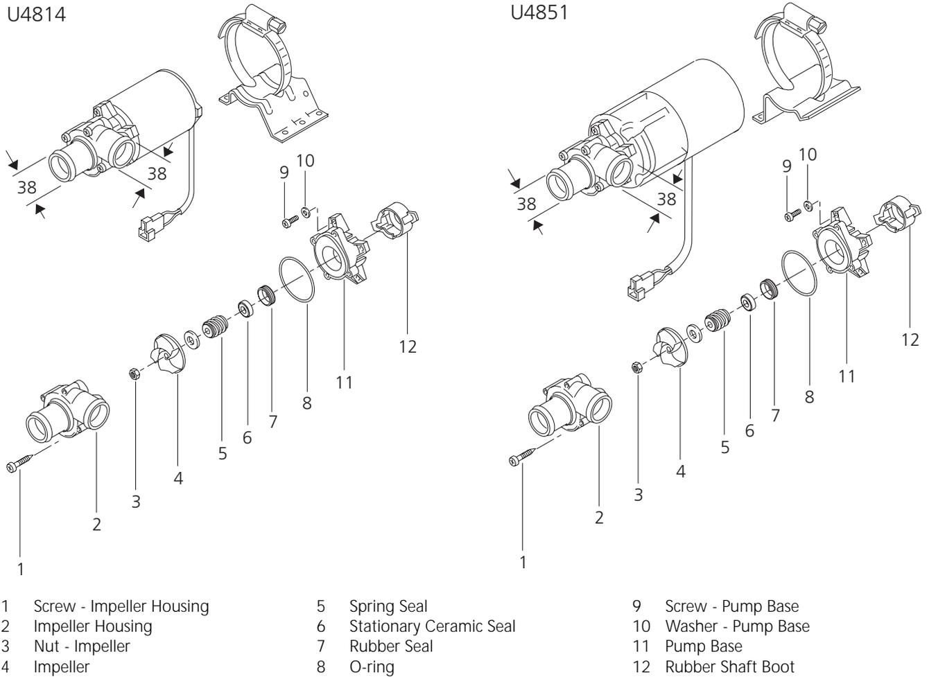
Figure 54: U4814 and U4851 Circulation Pump - Exploded View
