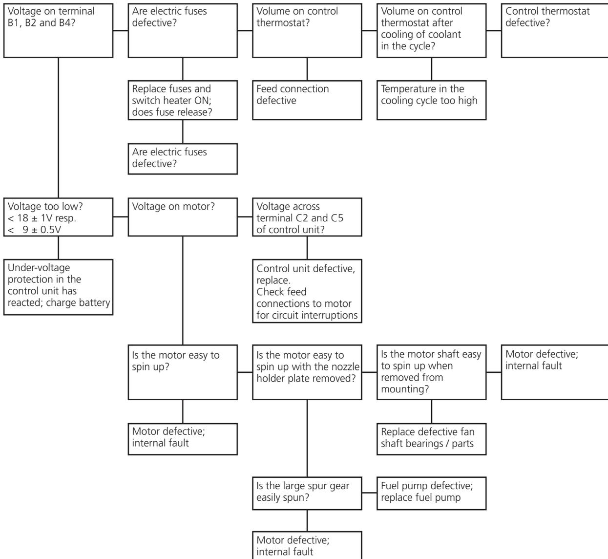
5.3.3 AFTER SWITCHING ON, THE HEATER SWITCHES OFF AFTER APPROX. 30 SECONDS ON FAULT
