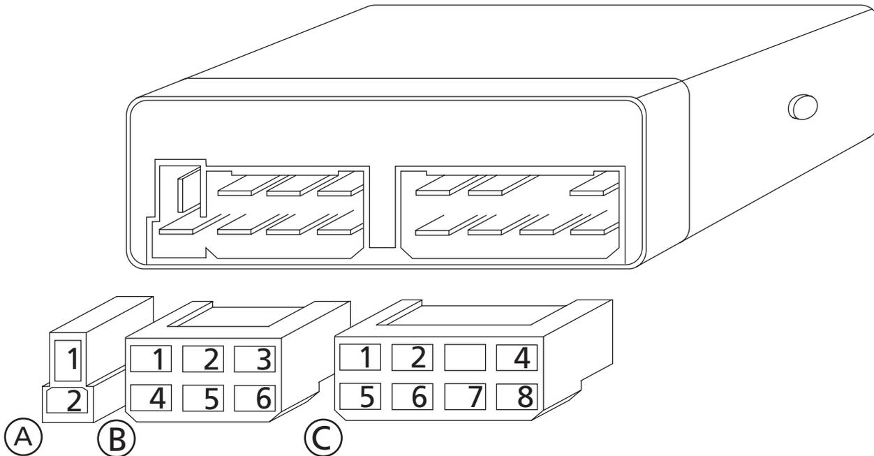
Figure 33: Control Unit - Identification of Terminals
