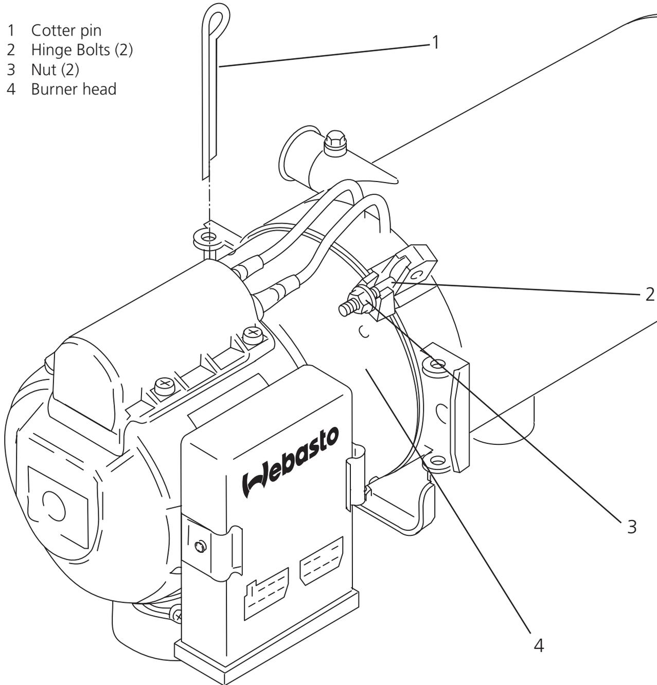
NOTE: Depending on the burner head direction of swing, the cotter pin may be located to the opposite side.
