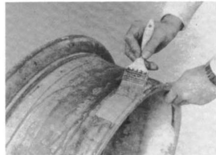
Paint rim by brush or spray with a fast-drying metal primer. Surfaces should be clean and dry prior to painting. Ensure that bare metal areas on outside or tire side of rim are covered. This is especially important on drop-center tubeless rims, because warm and sometimes moist air is in constant contact with the metal surface on the tire side of the rim.
