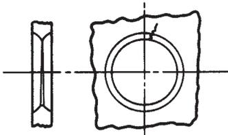
Crack originating from thin
