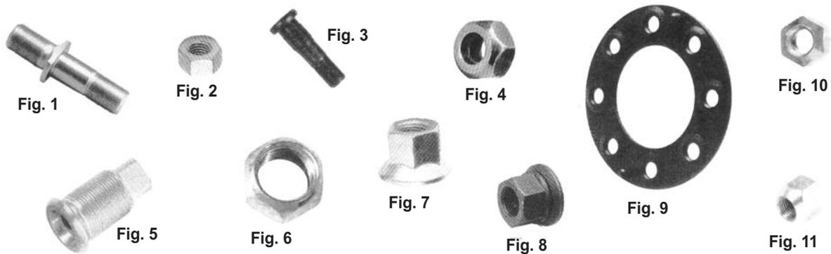
On front stud mount wheels, an outer cap nut (**Fig. 4**) or (**Fig. 6**) is used. On stud mount rear dual wheel applications, the inner wheel is held in place by an inner cap nut (**Fig. 5**) and the outer wheel by an outer cap nut (**Fig. 6**).
