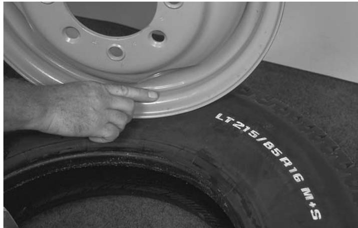
**⚠ WARNING:** Mounting a smaller diameter tire on a larger diameter rim/wheel (for example, a 16-inch tire on a 16.5-inch rim/wheel) can result in failure of the tire bead during mounting or airing. Mounting a larger diameter tire on a smaller diameter rim can result in unseating of the tire bead during operation. The tire may explode, striking a worker or bystander with deadly force. Check tire and rim/wheel diameter before starting to mount the assembly.
