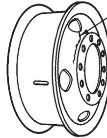
Cracks at disc nave
