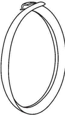
Sprung ring. Causes: Improper installation, or removal.
