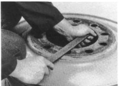
Wheel disc mating surfaces must be kept flat. Remove any metal projections, burrs at the stud hole chamfers and paint buildup.
