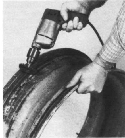
Bead seat areas of rim should be free of rust and rubber deposits. This is especially important for drop-center tubeless rims, because the bead seat is the air-sealing element.
