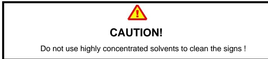
The different components of the EDSS can be cleaned with a moist towel. We recommend the use of a mild soap for the casing and a domestic glass cleaner for the acrylic window of the outside Rear Sign. Do not use highly concentrated solvents that would damage the acrylic window.
