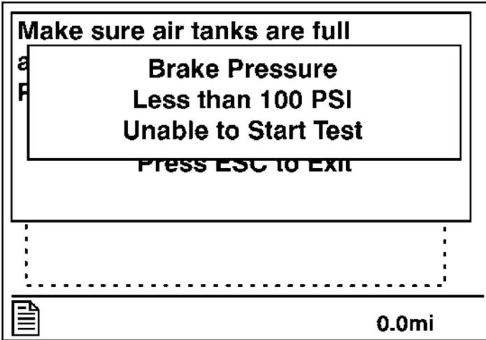
2. When the system is ready to be checked, the following screen displays. Press Enter to begin the test.
