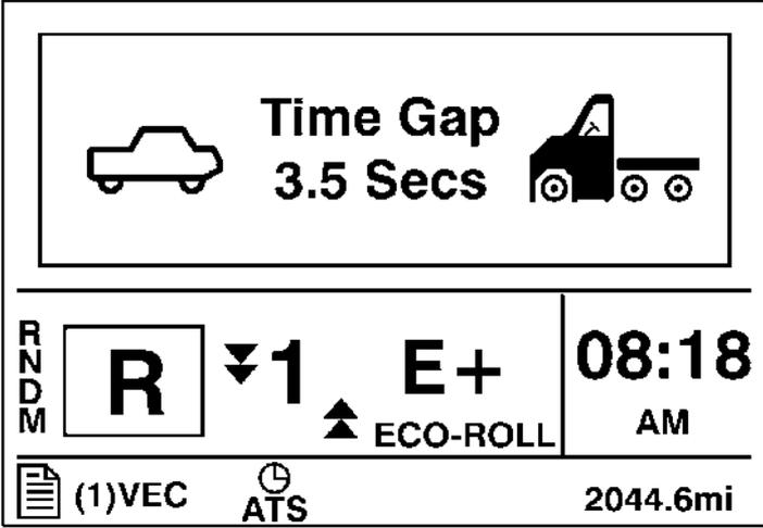
3. If the VEC detects that the vehicle is within a certain distance that a vehicle collision is eminent, driver intervention is required. The following screen displays.
