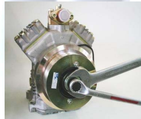
Take off from compressor
