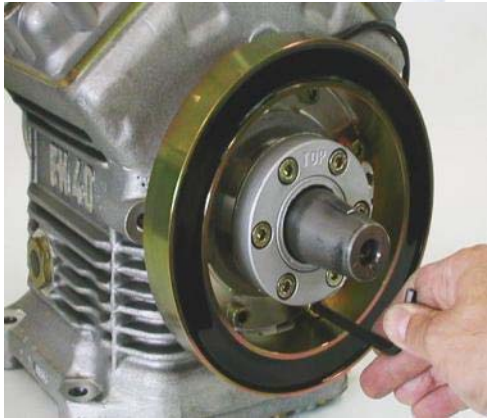
Mounting of the coil (Torque: Bitzer 25Nm, Bock 34Nm)
