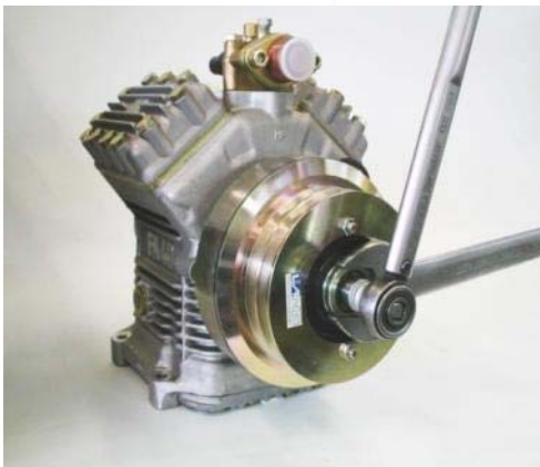
Fixing of the clutch (Torque: 60-80 Nm)
