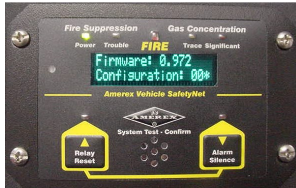
Figure 4.6.1b—Displays the current Software Revision Level (May be different than shown here)
