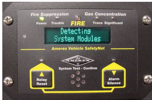
Figure 4.6.1d—Identifies Number of Modules Found (Driver, Detection, Detection Release, and/or Release Module)
