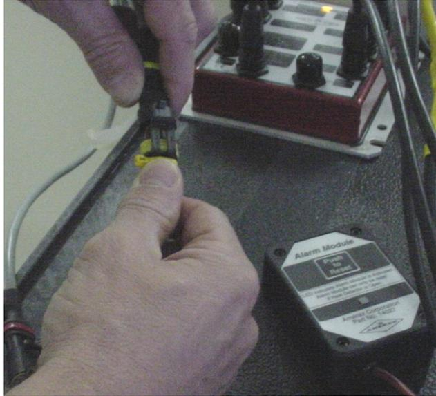
Figure 2 - Attach Alarm Module if necessary
