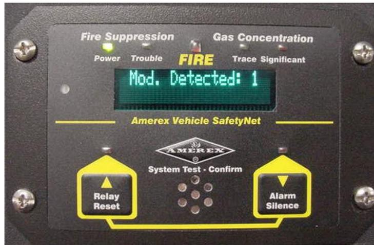
Figure 26- SafetyNet recognizes new Module in the Configuration,
