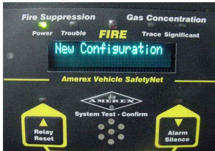
Figure 24 - The SafetyNet system acknowledges the New Configuration,
