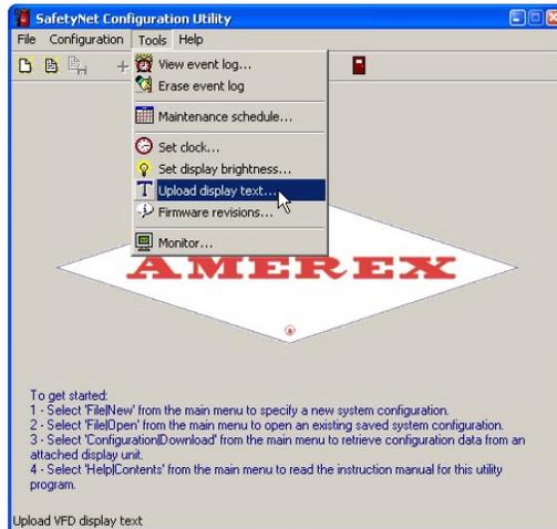
Figure 17 - Select Upload display text to modify Operator Display text
