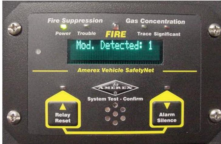
Figure 5 - Only (1) module has been detected
