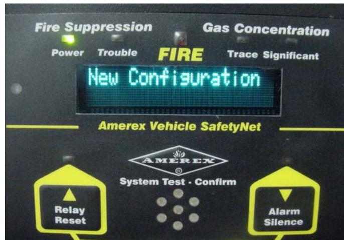
Figure 17 - The SafetyNet system acknowledges the New Configuration
