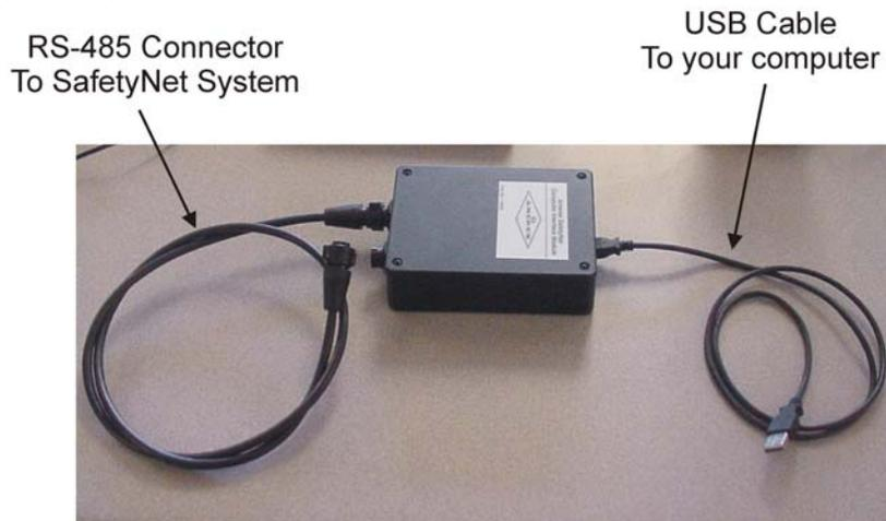
Figure 1 – P/N 16609 SafetyNet Computer Interface Module
