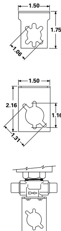
Installation for Types A3, E3\*, E5\*, B6, E6\*, W6, E8\*, B9, E9\*, B10, E10S1\*, E10S2, B14, E14, W14, B19, E19, W19, B25, E25, W25, Series Solenoid Valves.
