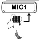
Whenever any one of the microphone inputs is activated, the control head switches over to the P.A. function. The P.A. has priority over all other channels. When activated, all other audio is muted. The P.A. system may be activated even when the control unit's Power button is not activated. While the P.A. system is active, the sound levels and tone (of the P.A. system) may be adjusted. These levels will only affect the P.A. system. Driver's Mic has priority over the Wireless Mic.
