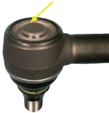
Assembly group 33 - deep cover, low height maximum of 0.5 mm deflection
