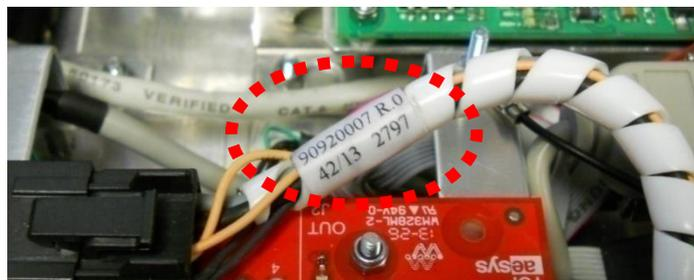
**Figure 8-2:** example of code and release imprinted on a wiring cable
