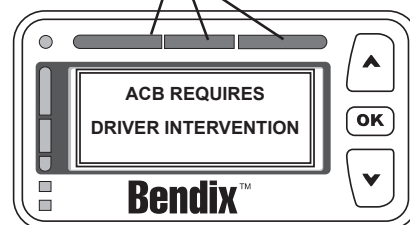
Figure K14 – Impact Alert Text and Light Pattern as Seen on the Bendix DIU
