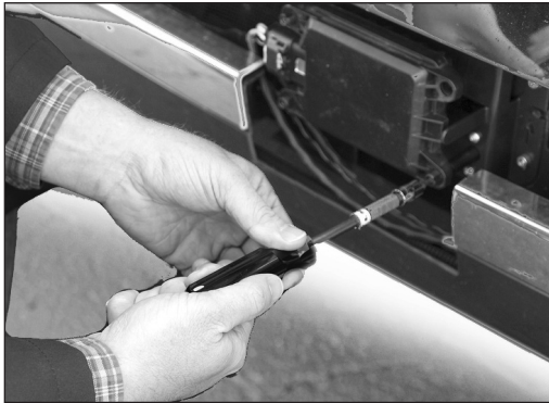
A technician makes an adjustment to the lateral alignment standoff.
