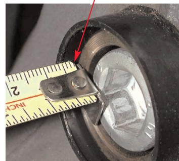
FIGURE 3: Worn Pads 4 to 8mm (.157" to .315")
