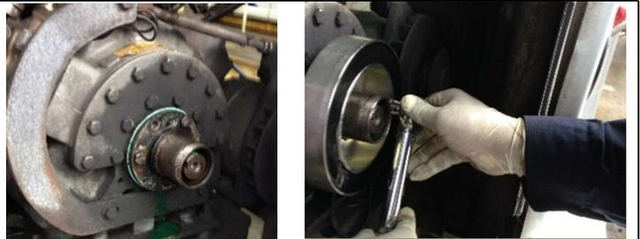
3. Slide the pulley on the hub and torque the bearing retaining nut with tool 20-294, noting the torque required to seat the bearing against the hub. After the bearing seats, tighten the nut to 50 lbs-ft GREATER than the bearing-seating torque.
