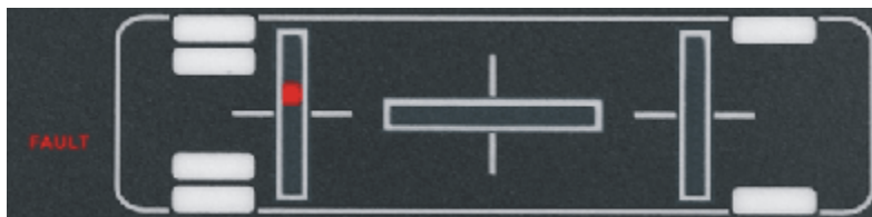
2. Short circuit in rear left Travel valve
