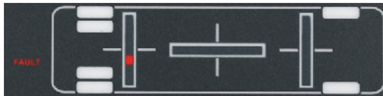
4. Short circuit in rear right Raise valve
