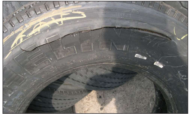
Fatigue Rupture or “Zipper”
