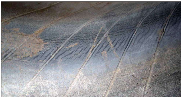
EFFECT: Inner Liner Marbling - Creasing CAUSE: Underinflation
