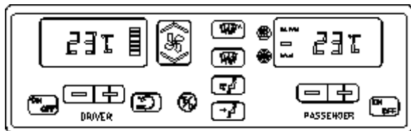
CENTRAL HVAC SYSTEM CONTROL MODULE
