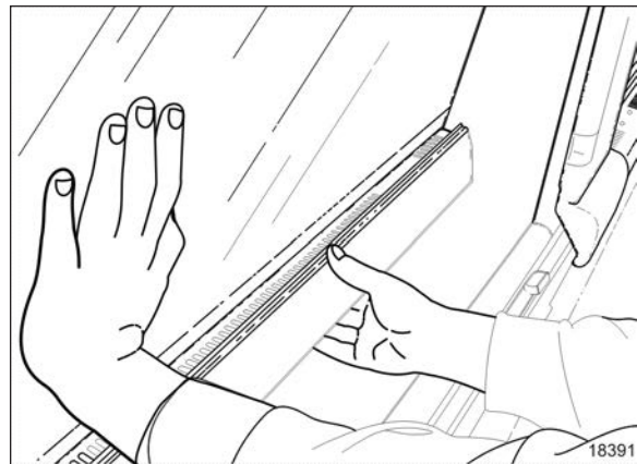
FIGURE 16: EMERGENCY WINDOW OPENING
