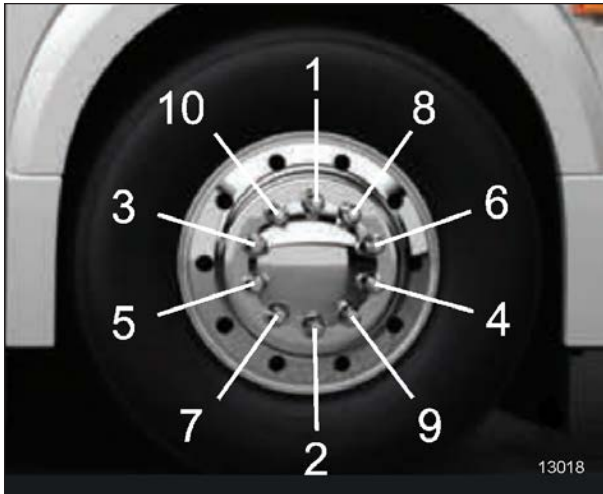
FIGURE 12: TIGHTENING SEQUENCE
