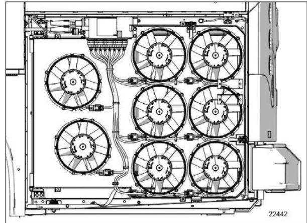
FIGURE 15: RADIATOR DOOR OPENED (FAN SHROUD NOT SHOWN)
