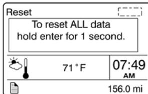
When the Reset Trip Data menu is open, pressing and holding down the Enter ↵ button for 1 second resets the functions listed below. This function will permit to the system to calculate new value from the point of resetting.
