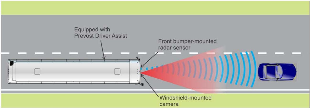
FIGURE 28: PREVOST DRIVER ASSIST™ SYSTEM USES A CAMERA AND RADAR SENSOR
