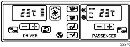
FIGURE 22: CONTROL UNIT FOR HIGH CAPACITY CENTRAL HVAC SYSTEM
