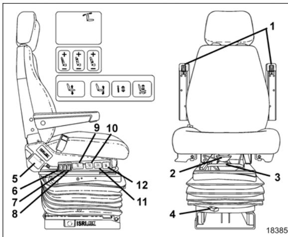
FIGURE 2: PNEUMATIC DRIVER'S SEAT
