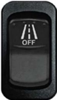
FIGURE 29: LDW ENABLE/DISABLE SWITCH
