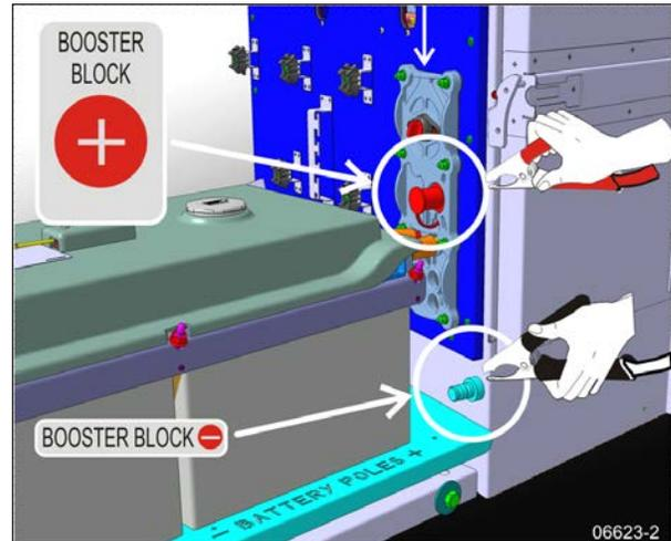
**FIGURE 4: BOOSTER BLOCK TERMINALS LOCATION (X3 SERIES)**
