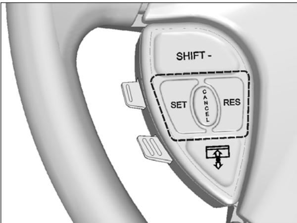
**FIGURE 27: CRUISE CONTROL BUTTONS**
