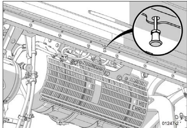
FIGURE 8: AFTERTREATMENT ACCESS DOOR LATCH
