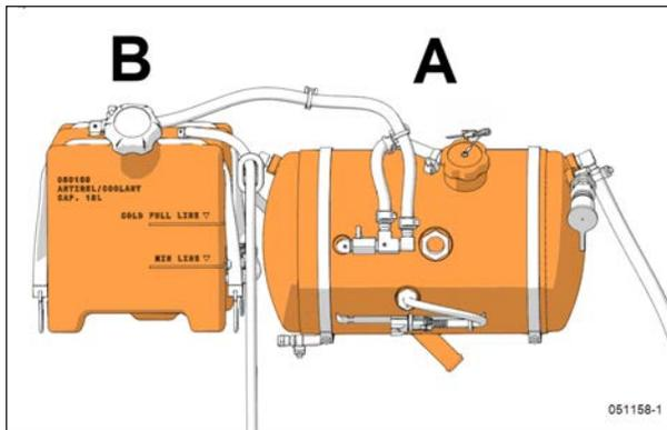
Check the coolant level into the recovery tank (B) when the engine is cold (ambient temperature).
