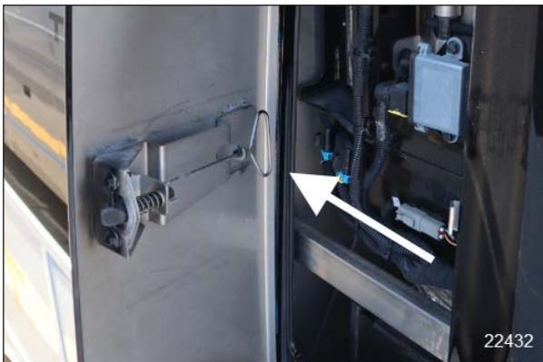
FIGURE 17: SCR ACCESS DOOR HANDLE
