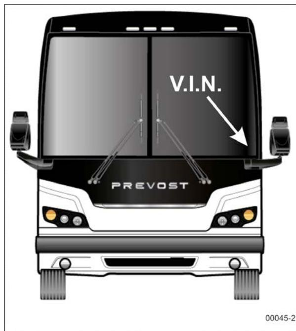
FIGURE 9: VEHICLE IDENTIFICATION NUMBER (X3 SERIES)
