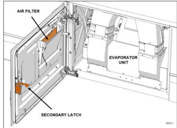
FIGURE 26: EVAPORATOR COMPARTMENT
