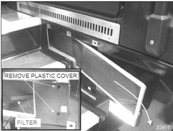
**FIGURE 21: REMOVING DRIVER'S SECTION AIR FILTER**
