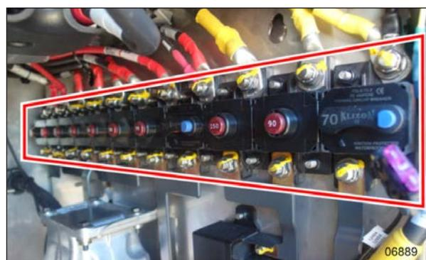
**FIGURE 12: MAIN CIRCUIT BREAKERS IN MPC (TYPICAL)**
