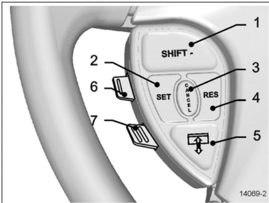
FIGURE 7: LEFT STEERING WHEEL CONTROLS
