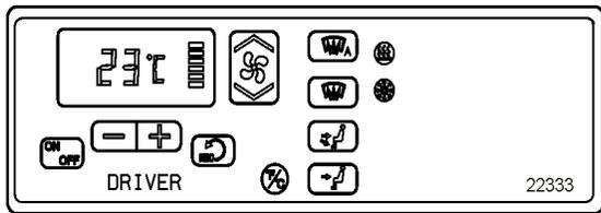
FIGURE 23: CONTROL UNIT FOR DRIVER'S HVAC SYSTEM
