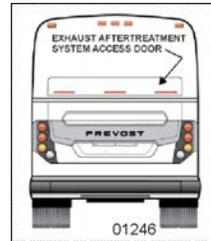
The engine door must be open before opening the exhaust aftertreatment system access door. To open the access door, pull down the latch release knob.
