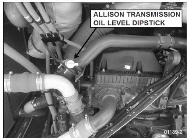
FIGURE 3: ENGINE L. H. SIDE (X3 SERIES)
