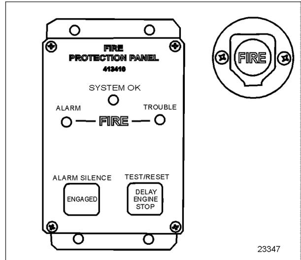
FIGURE 26: AFSS PANEL & MANUAL ACTIVATION SWITCH
