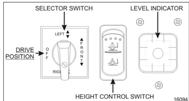
FIGURE 13: LEVEL LOW SYSTEM CONTROLS
