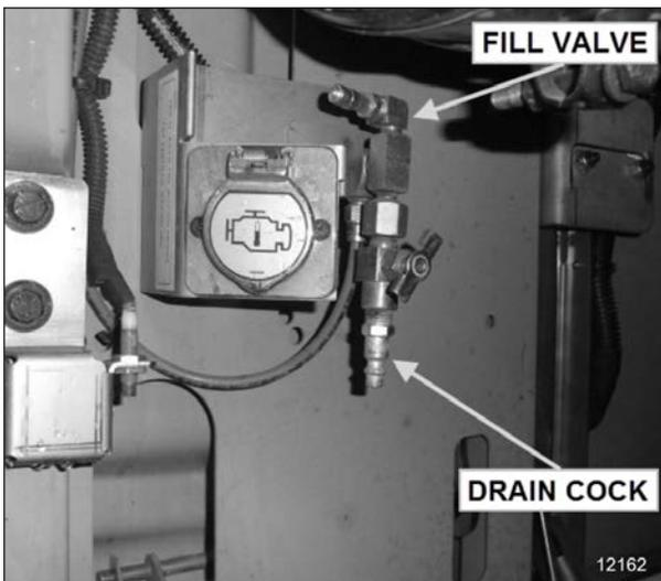
FIGURE 10: ENGINE COMPARTMENT FILL VALVES
