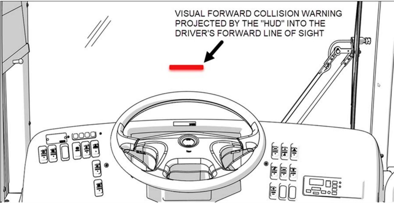
FIGURE 30: HEAD-UP DISPLAY PROJECTED VISUAL WARNING
