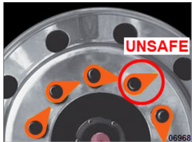
FIGURE 15: LOOSE WHEEL NUT INDICATORS - UNSAFE DRIVING CONDITION
