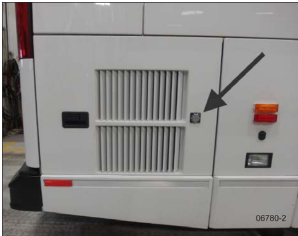
FIGURE 28: BATTERY CHARGER 120-VOLT CONNECTOR
