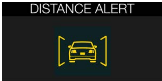
FIGURE 49: FOLLOWING DISTANCE ALERT WARNING POP-UP
