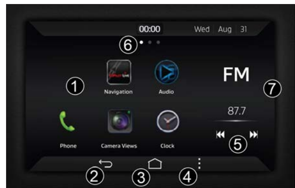
FIGURE 15: SECONDARY INFORMATION DISPLAY (SID) HOME PAGE NO.1
