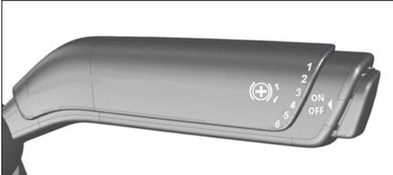
FIGURE 29: TRANSMISSION RETARDER CONTROL STALK
