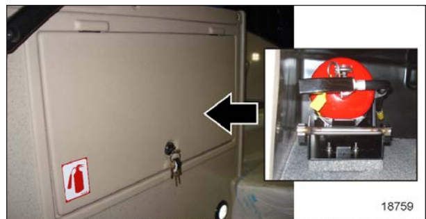
FIGURE 8: A DECAL INDICATES THAT A FIRE EXTINGUISHER (OPTION) IS LOCATED IN THE DRIVER'S PERSONAL COMPARTMENT
