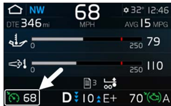
FIGURE 39: CRUISE CONTROL SET SPEED CONFIRMATION & CURRENT SET SPEED DISPLAYED IN THE SYSTEM STATUS ZONE
