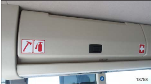
FIGURE 9: A DECAL INDICATES THAT A FIRE HATCHET, A FIRE EXTINGUISHER AND A FIRST-AID KIT ARE LOCATED IN THIS OVERHEAD COMPARTMENT
