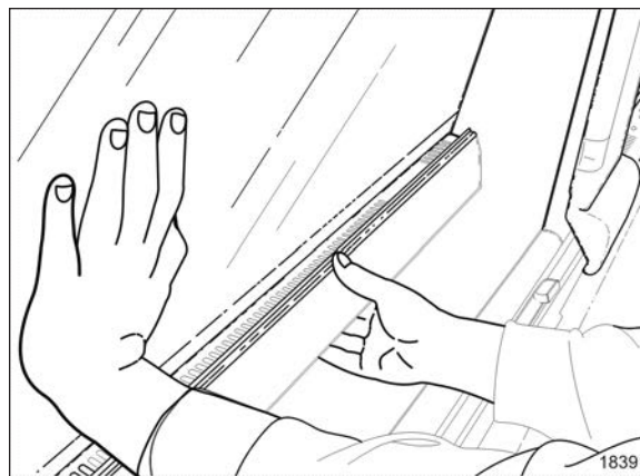
FIGURE 14: EMERGENCY WINDOW OPENING
