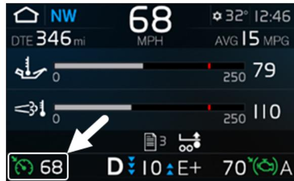
FIGURE 40: CRUISE CONTROL SET SPEED CONFIRMATION & CURRENT SET SPEED DISPLAYED IN THE SYSTEM STATUS ZONE
