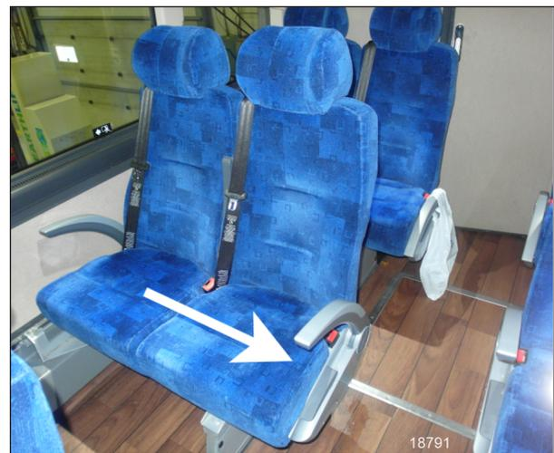
**FIGURE 10: PULL TO UNLOCK THE ROTATION**
