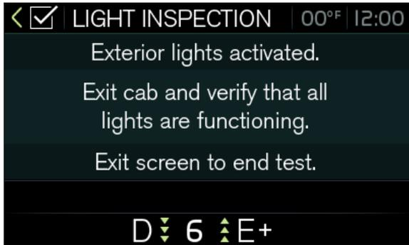
To exit test, press APPLICATION TRAY / BACK button, then select REMOVE FORCE AND END TESTS and press ENTER / SELECT button.
