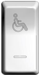
Supply electrical power to the wheelchair lift system by pressing down on the rocker switch. Refer to Other Features for instructions on operating the wheelchair lift.
