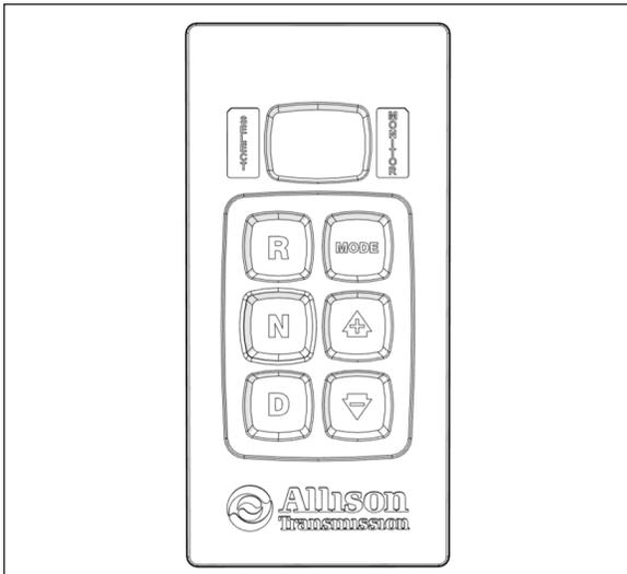
FIGURE 6: TRANSMISSION CONTROL PAD
