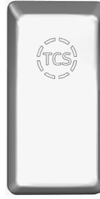
On certain road conditions, it may be useful to retard the intervention of the traction control system TCS during vehicle acceleration. The Mud/Snow function allows greater engine power and more wheel spin during TCS operation. This function may be helpful to set the vehicle in motion on iced roads, for example.
