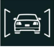
FIGURE 47: FORWARD VEHICLE DETECTED STATUS PICTOGRAM (WHITE)
