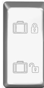
This system enables locking all baggage compartment doors by pressing the switch forward. To unlock, press the switch rearward.
