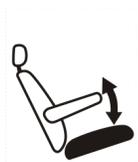
To lower or raise the seat's front section, pull the handle #3 up and push or pull the seat cushion.
