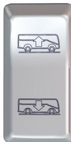
Press and hold this rocker switch to raise or lower the coach about 4 inches (100 mm). Release the rocker switch to return the coach to the normal driving height.
