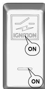
The main electrical shut-off switch is in the ON position and the ignition switch is flipped on.
