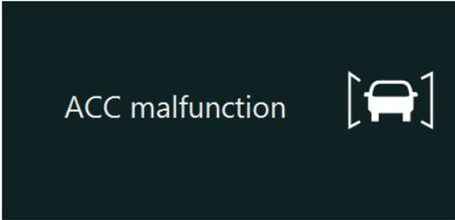
For the proper functioning of the system, the radar must be perfectly aligned and not blocked. If a radar fault condition is detected, one of the following pop-up messages will show in the DID.
