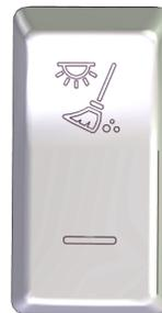
Press this rocker switch to turn on the interior lighting in the most appropriate mode when cleaning the interior. Prior to do so, connect the vehicle to a battery charger.
