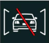
FORWARD VEHICLE DETECTED - MISSING/ERROR STATE pictogram
