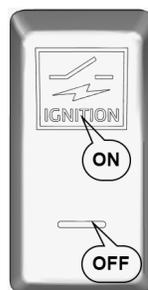
State: vehicle in wake up mode. Pictogram ON and LED OFF.
