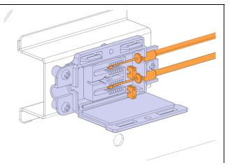
9. Remove the splitter and screws (3x). Keep the splitter and hardware for reuse.
