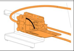
7. Remove the cable from the splitter and discard.
