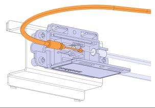
8. Remove the clips (2x) and then remove the two cables from door latches.
