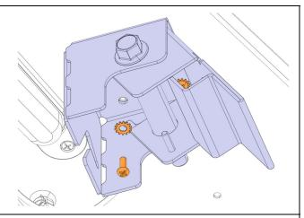
5. Remove the cable ties that secure the cable.
