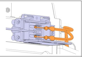
5. Secure the cables with the two clips. Do not insert the clips too tightly on cables.
