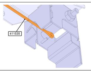
4. Install the new rod 411535 in the splitter. 411535 5. Secure the rod 411535 on the handle with one nut (1x) and one spacer (1x). 411535 6. Install cable tie mount 504013(1x) with rivet 504379(1x). 504379 504013
