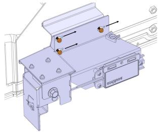
3. Tighten the screws to a torque of 20 lb-in.
