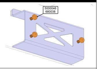
2. Slide the new assembly on the screws installed in the previous step.
