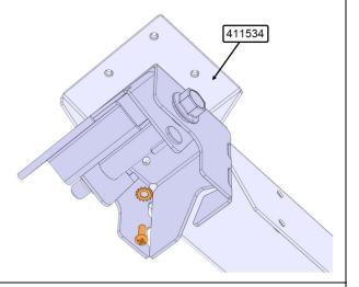
2. Reinstall the splitter on the new support 411534 with three screws (3x).
