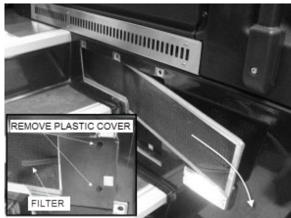
FIGURE 26: REMOVING DRIVER'S SECTION AIR FILTERS
