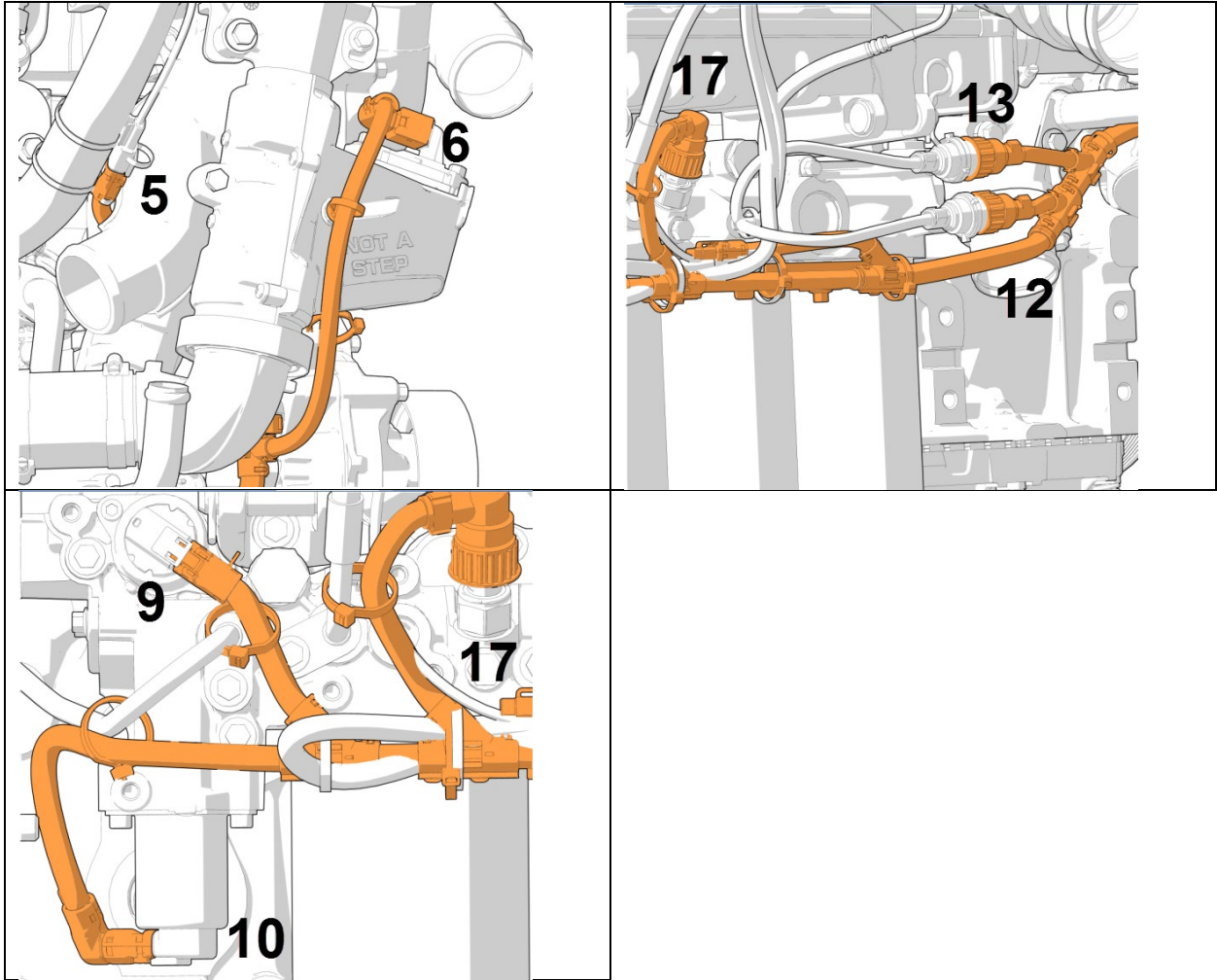
FIGURE 2: ENGINE HARNESS CONNECTION POINTS
