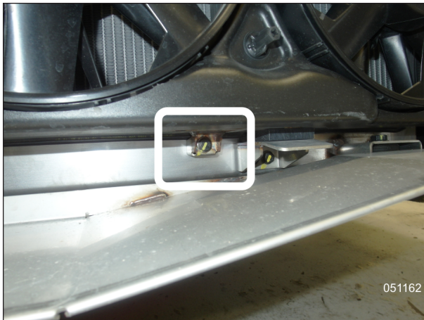
FIGURE 11: FAN SHROUD TOP & BOTTOM HOLD-DOWN SCREWS
