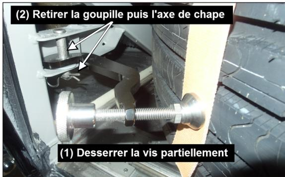
FIGURE 13: RETRAIT DE LA ROUE DE SECOURS
