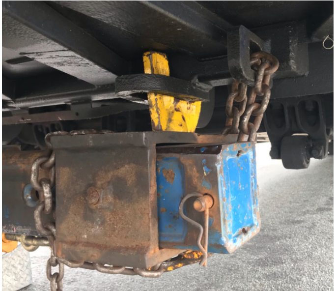
Figure 41: DOB BUS NUMBER SERIES 1300-1629 & 1630-1879 CHOKE CHAINS ROUTING
