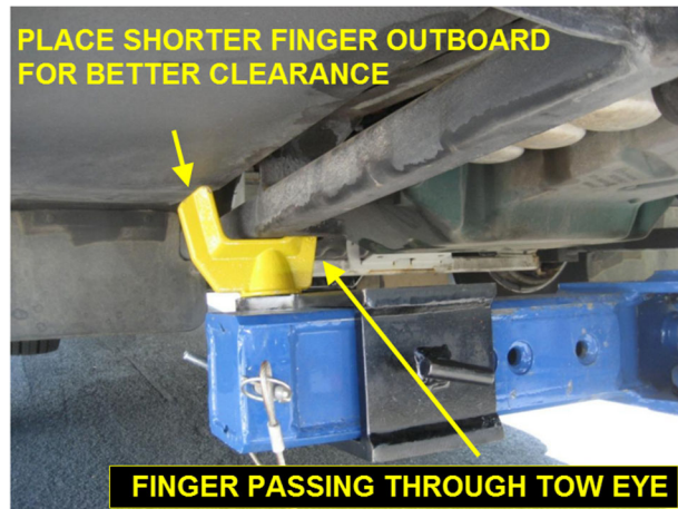
Figure 69: PROPER LOCATION WHEN LIFTING THE SIDE-MEMBERS – ON THIS PICTURE, THE BUS IS EQUIPPED WITH REAR TOW EYES
