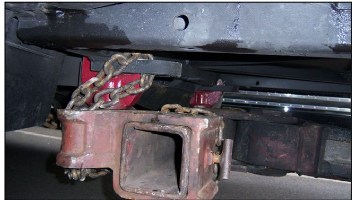
Figure 40: DOB BUS NUMBER SERIES 2400–2489 & 2490–2789 CHOKE CHAINS ROUTING
