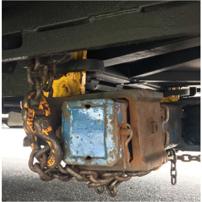
Figure 43: : DOB BUS NUMBER SERIES 1300-1629 & 1630-1879 CHOKE CHAINS ROUTING
