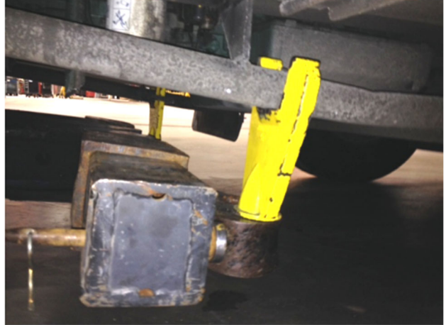
Figure 68: PROPER LOCATION WHEN LIFTING THE SIDE-MEMBERS
