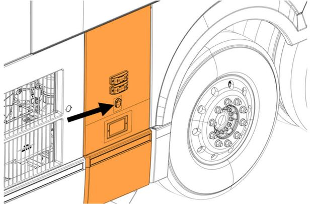
2. Remove the decal of the rear junction box components.
