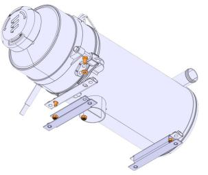
20. Remove the air intake of the new heater 870289.
