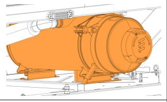
19. Unscrew the supports (2x) from the heater, keep the supports (2x), the screws (4x) and the washers (4x) and discard the nuts (4x).
