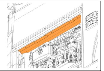
56. Connect the new timer harness 0610675 to connector **C430** of the left consol harness.
