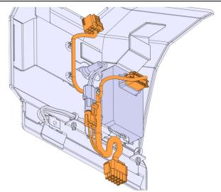
56. Install the new cover 870253 on the consol in the hole for the heater timer.
