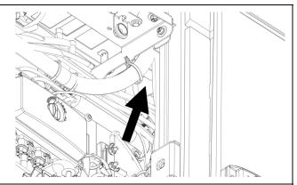
62. Connect the connector **C\_A11B** of the heater to timer CAN harness 0610673 to connector **A11** of consol harness 0600216.
