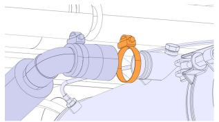
29. Reinstall the exhaust pipe with U-bolt clamp.
