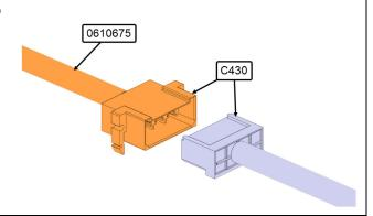
57. Connect the connector **C\_A11B** of the heater to timer CAN harness 0610673 to connector **A11** of timer harness 0610675.
