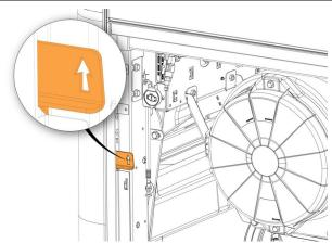
3. Pull the engine compartment door out and up to open.
