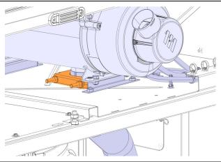
30. Secure the exhaust pipe bottom with the screw and the new washer 5001848.
