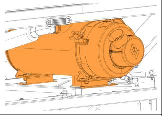
24. Secure the new heater assembly with the screws (4x) and the new washers 5001848 (4x) on the structure.
