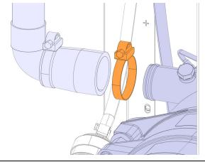
26. Reinstall the exhaust with U-bolt clamp.
