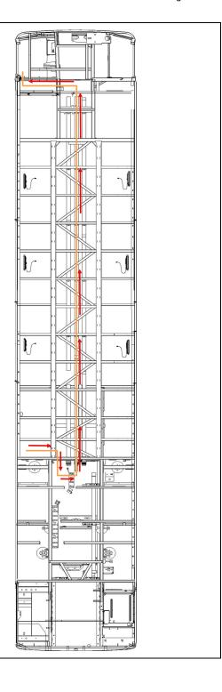
39. Connect the connector **A10.A3** of the heater to timer CAN harness 0610673 to heater position **2**.
