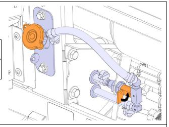
7. Locate the drain cock at the radiator water pipe.
