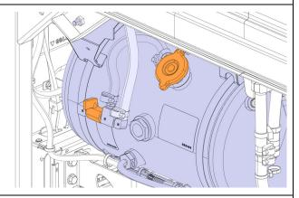
6. Locate coolant extractor fitting under the vehicle
