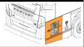
2. Lift the release lever to unlatch the engine compartment door.
