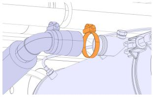
16. Unscrew the clamp and disconnect the outlet hose.
