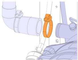
15. Unscrew the clamp and disconnect the outlet hose.
