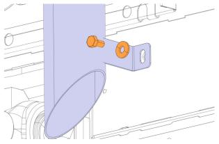
11. Unscrew the U-bolt clamp and remove the exhaust.
