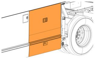
33. Drill a hole to  $\emptyset$  3/8" in baggage panel. 6.6" Ø 3/8" 34. Drill a hole to Ø 2 1/4" in baggage panel. Ø 2 1/4" 35. Install the 400632 flange and drill three Ø .129 holes (No. 30 drill bit) using the existing flange holes as a template.
