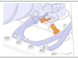
15. Unscrew the clamp and disconnect the inlet hose.
