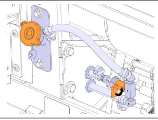
7. Locate the drain cock at the radiator water pipe.
