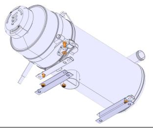
20. Remove the air intake of the new heater 870289.
