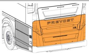
4. Press the release lever and push the DPF access hatch up until it locks in place.
