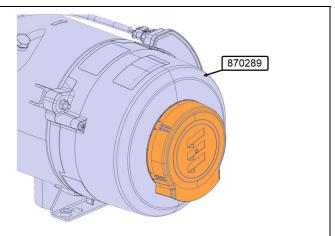
21. Install the new air intake 870295 on the new heater 870289.
