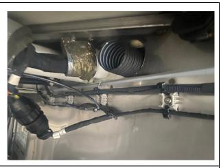
32. Connect the hose 503031 to the heater air intake with clamp 504024.
