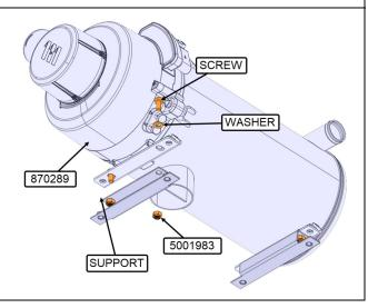
23. Install the new heater assembly.
