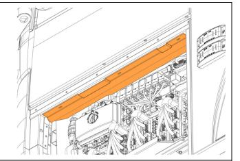
53. Connect the new timer harness 0610675 to connector **C430** of the left consol harness.
