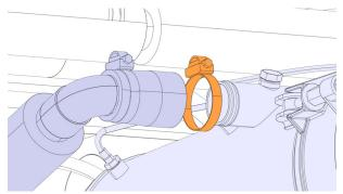
29. Reinstall the exhaust pipe with U-bolt clamp.
