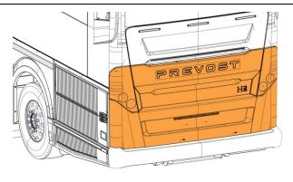
4. Press the release lever and push the DPF access hatch up until it locks in place.
