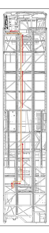
46. Connect the connector **A10.A3** of the heater to timer CAN harness 0610673 to heater position **2**.
