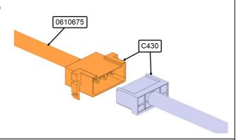
54. Connect the connector **C\_A11B** of the heater to timer CAN harness 0610673 to connector **A11** of timer harness 0610675.
