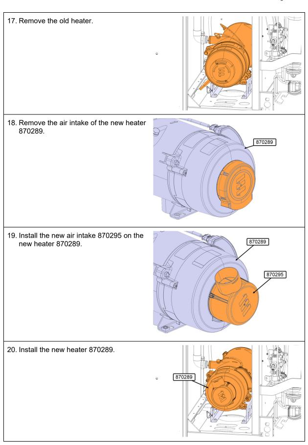
21. Secure the new heater 870289 with the screws (4x) and the new washers 5001848 (4x) on the support.
