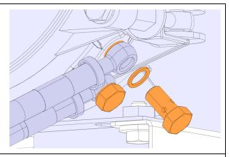
14. Unscrew the clamp and disconnect the inlet hose.
