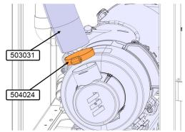
33. Secure the hose 503031 on existing hose with the dual swivel saddle spacers 504751 (3x) and the cable ties 504016 (6x).
