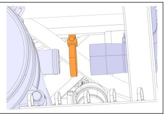
17. Unscrew the heater assembly, keep the screw (4x) and discard the washer (4x).
