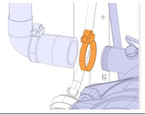
26. Reinstall the exhaust with U-bolt clamp.
