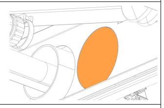
30. Run the hose 503031 through the hole and reach the preheater compartment.
