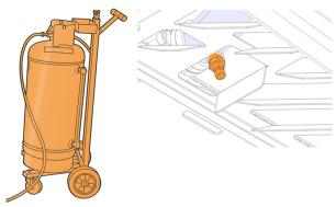
55. Disconnect the coolant extractor and reinstall the protection cap.
