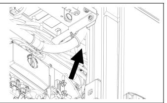
59. Connect the connector **C\_A11B** of the heater to timer CAN harness 0610673 to connector **A11** of consol harness 0600216.
