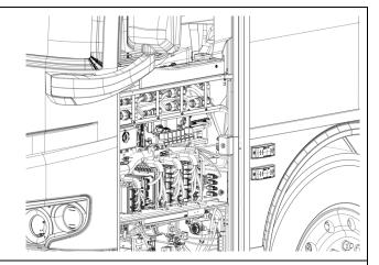
45. Connect the new timer harness 0610675 to connector **C430** of the left consol harness.
