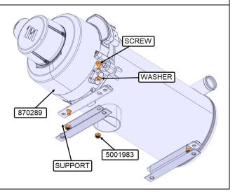
23. Install the new heater assembly.
