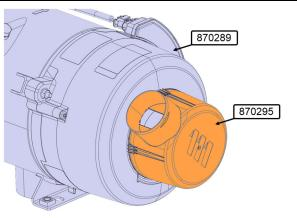
22. Install the supports (2X) on the new heater 870289 with the screws (4x), the washers (4x) and the new nuts 5001983 (4x).
