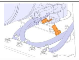
15. Unscrew the clamp and disconnect the inlet hose.
