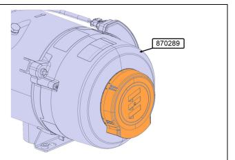
21. Install the new air intake 870295 on the new heater 870289.
