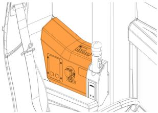
48. Disconnect connector **C430** of the consol harness from the front junction box main harness.
