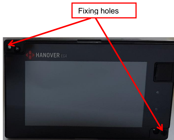
Figure 7 - diagram showing the 2 fixing holes
