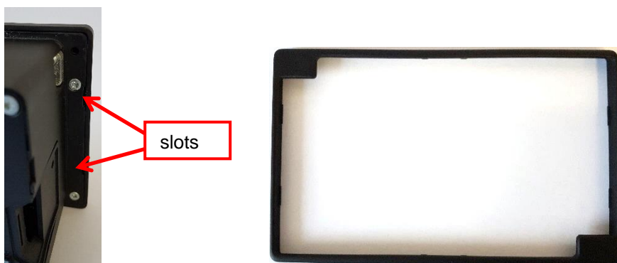
Figure 5 - diagrams showing the front bezel removed using the slots
