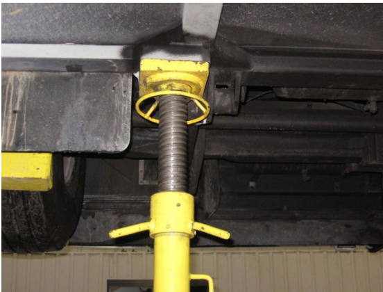
FIGURE 17 : JACK STAND AT CHASSIS HOISTING RECEPTACLE - AFT OF FRONT AXLE, ROAD SIDE
