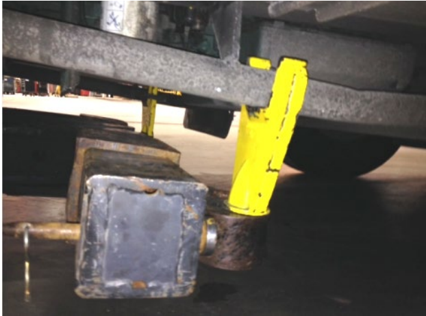
FIGURE 61 : PROPER LOCATION WHEN LIFTING THE SIDE MEMBERS
