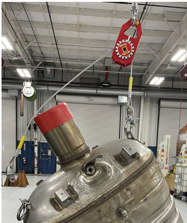
Oberg tilt lift 2,000 lbs. Capacity – special lifting tool available in Service Centers use with half-inch ratchet or half-inch breaker bar
