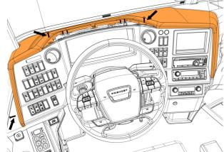
5. Unplug the four connectors at the back of the instrument cluster.
