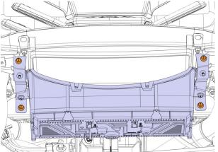
14. Plug the four connectors at the back of the instrument cluster.
