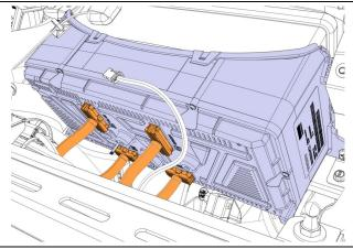
15. Reinstall the dashboard cover and fasten it with the screws (3x).
