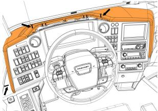
16. Reinstall the instrument panel cover with the screws (2x).
