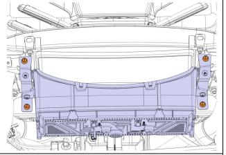
8. Remove the instrument cluster with the brackets from the dashboard.
