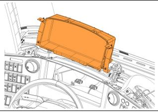
13. Fasten the cluster assembly to the dash-board with the bolts (4x).
