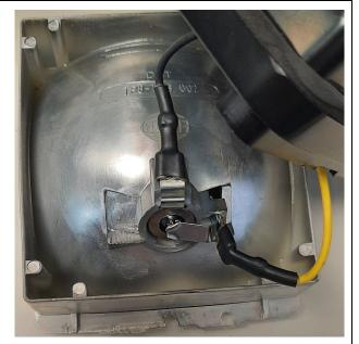
14. Place the reflector in the housing, reinstall the lens and tighten with new screws **502664** (2x).
