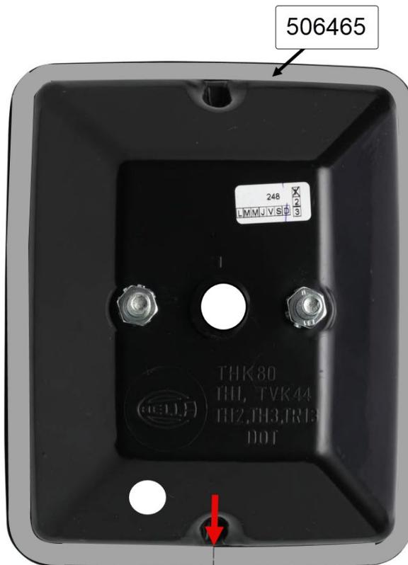
7. Install the grommet in the new drilled hole.
