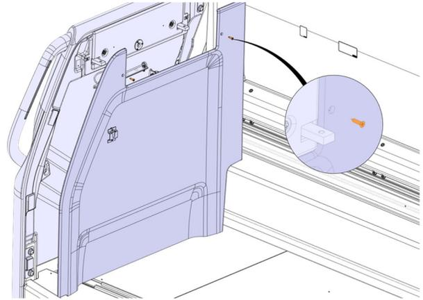
7. Reinstall the shelf with the nuts (2x) and the washer (2x).
