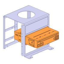
16. Make a rectangular cut at the back plate of the support to accommodate the HDMI cable connection.
