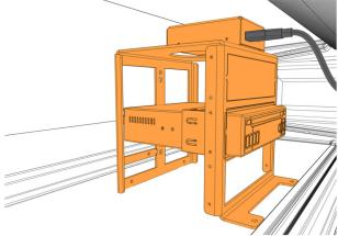
33. Connect the connector **C** "OUT" of preamplifier 7775435 to the audio harness **901565**.
