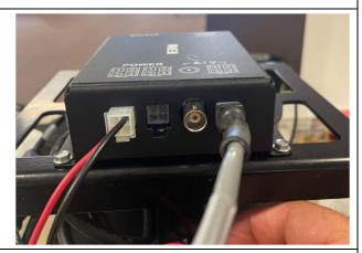
31. Plug connector **B** of the pre-amplifier 7775435 into the power input at the rear of the DVD player.
