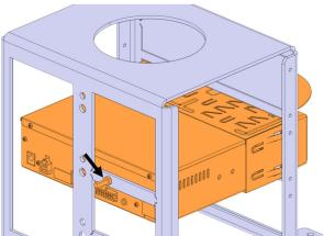
21. Connect cable 7775434 to the HDMI converter input.
