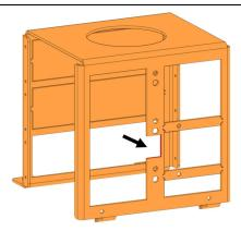
17. Drill four (4) holes of 9/64-inch diameter at the top of the support for the HDMI converter 901567.
