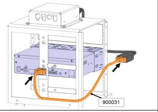
23. Secure the cables with cable-ties (2x) 504637.
