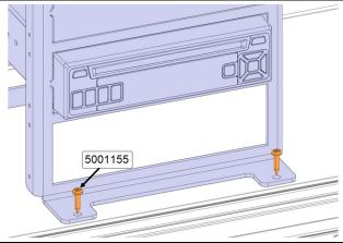
42. Secure the rear of the support using the p-clamp and new screw 5001155.
