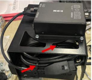
24. Remove the 2-pin power connector A of the pre-amplifier 7775435, to replace it with a 4-pin connector.
