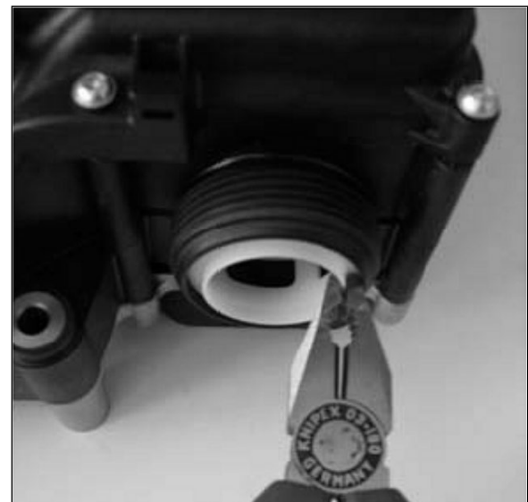
FIGURE 13 : PUMP ASSEMBLY FILTER ELEMENT
