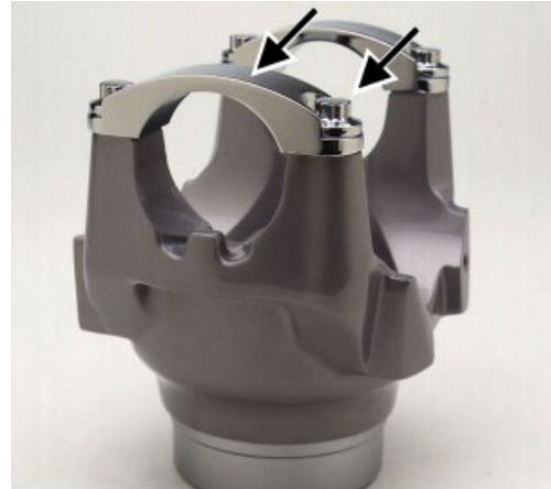
FIGURE 2: COLD FORMED BEARING RETAINER AND BOLTS AS USED ON PREVOST VEHICLES
