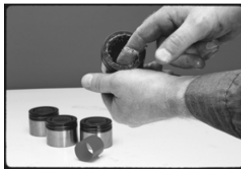
FIGURE 27: GREASING BEARING CUP
