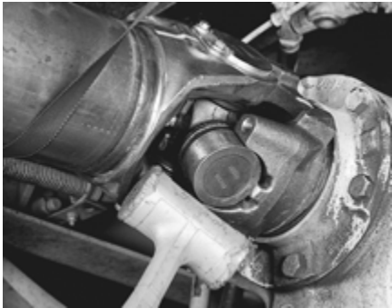
FIGURE 13: UNSEATING BEARING CUP ASSEMBLIES
