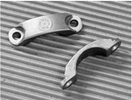
FIGURE 12: COLD FORMED BEARING RETAINERS
