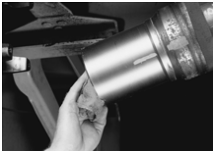
FIGURE 22: CLEAN GREASE FROM SPLINE SLEEVE
