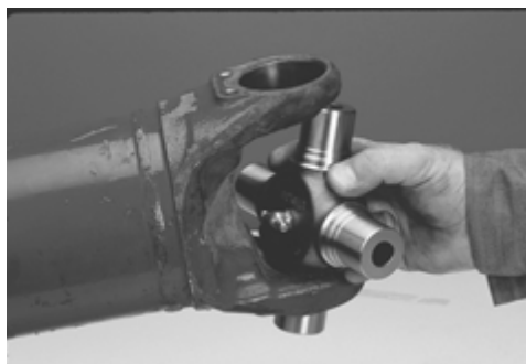
FIGURE 28: POSITION THE JOURNAL CROSS INTO THE YOKE CROSS HOLES WITH THE GREASE ZERK FITTING INWARD TOWARD TUBING
