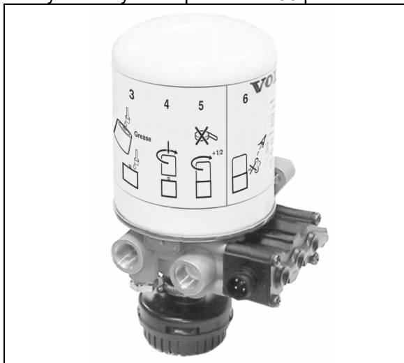
FIGURE 12: AIR FILTER DRYER
