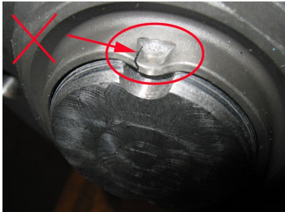
FIGURE 26: BROCKEN OR TORN LIP – REJECTED
