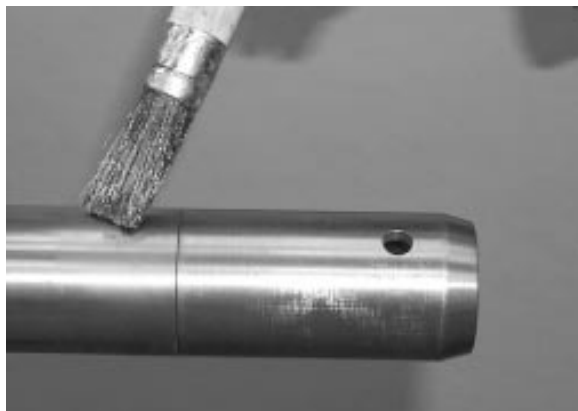
FIGURE 19: APPLY GLEITMO 805 GREASE
