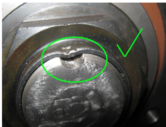
FIGURE 24: CORRECT - PREVENTS THE NUT FROM GETTING LOOSE
