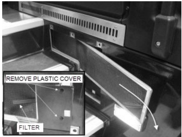
FIGURE 26: REMOVING DRIVER'S SECTION AIR FILTERS
