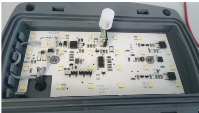
Pins 7 and 8 shorted(light dimmed all the time)
