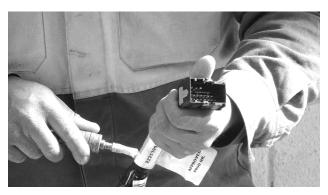
9) Use compressed air to blow away any metal shavings accumulated inside the connectors bracket.
