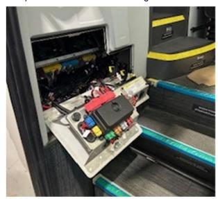
4) Unscrew and remove the cover plate over the connectors bracket.
