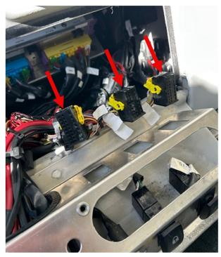
6) Remove the connector pin board from each interface connector housing.
